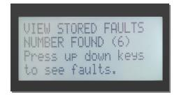
Pressing the **DOWN** button will display the first stored fault. In this case, an "Open Circuit" is indicated. Press the **DOWN** button again to display the next stored fault. Press the **UP** button to return to the previous fault.
