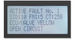
When the fault is displayed, press the SELECT key to view the manufacturer's repair notes.
